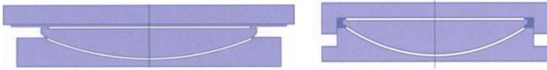
Figure 3. Fixed and moving friction pendulum bearing supports
